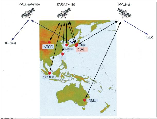
Fig.7 Current status of two-way satellite time/frequency transfer network in the Pacific Rim region
