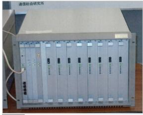
Fig.4 Multi-channel two-way satellite time/frequency transfer modem Equipment features two transmitting channels and eight receiving channels
